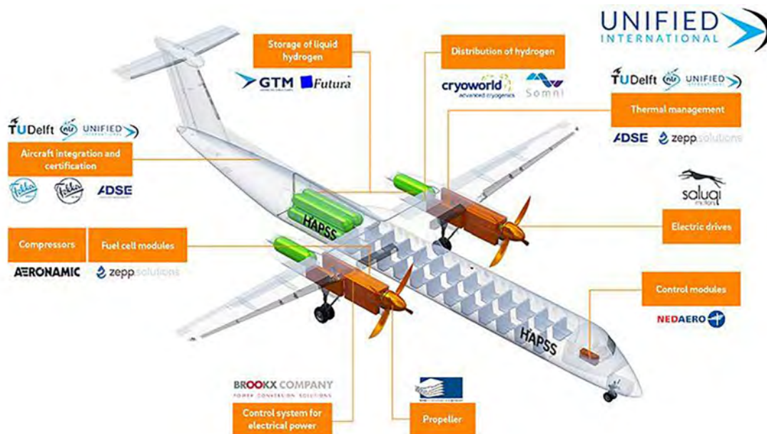
Figure 2.12: Fuel Cell/Battery Hydrogen Powered Propulsion System
